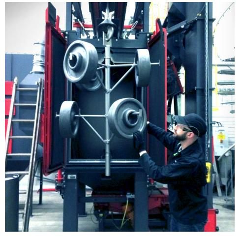
• Check abrasive quality, removing any large clusters which may have formed due to moisture.
