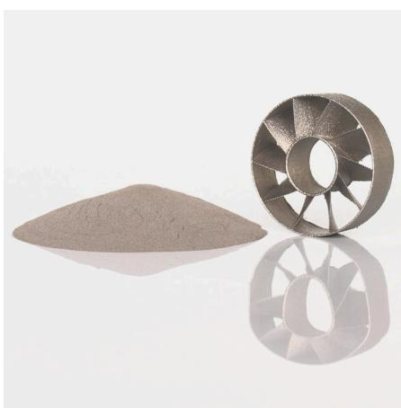
Through the development of centrifugal atomization technology, Ervin Technologies produces highly spherical metal powders. The Rapid Solidification Rate (RSR) technology enables the production of unique microstructures unattainable through some other atomization methods. The extremely high cooling rates from the RSR technology create fine-grained (nanometre-scale) and amorphous metals with uniform chemistry.
