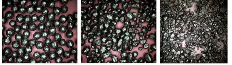
Amasteel Shot, Amasteel MG Grit and Amasteel HG Grit 500 kumlama döngüsü sonra
